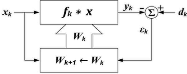
Fig 2. subband adaptive closed loop filtering
